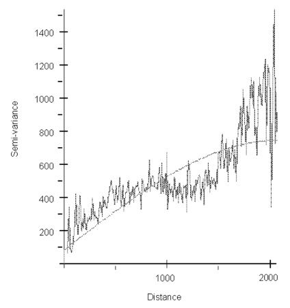
Figure 4. Example of an empirical variogram for the magnitude of the distortion field between two street centerline databases. The smooth curve shows the fitted variogram model.
