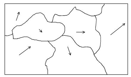
Figure 5: A 'patch' model of a distortion field, with discontinuities at patch boundaries (arrow lengths not to scale)
