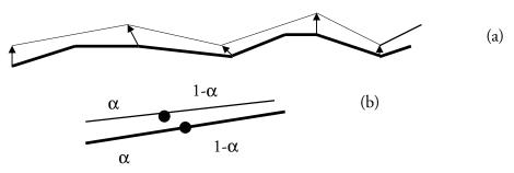
Figure 1: Matching points to estimate displacement: (a) matching well-defined points; (b) matching interpolated points based on distance along the line.
