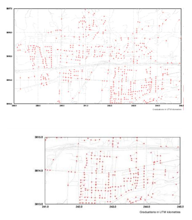
Figure 3: Distortion vectors computed by matching nodes between two commercial databases for part of Goleta, CA. The lower illustration is an enlargement of part of the upper.
